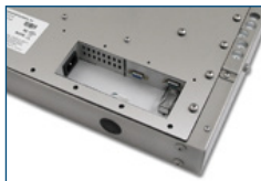
Opening to Internal Connectors
