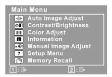
**NOTE:** All OSD menus and adjustment screens disappear automatically after about 15 seconds. This is adjustable through the OSD timeout setting in the Setup Menu
