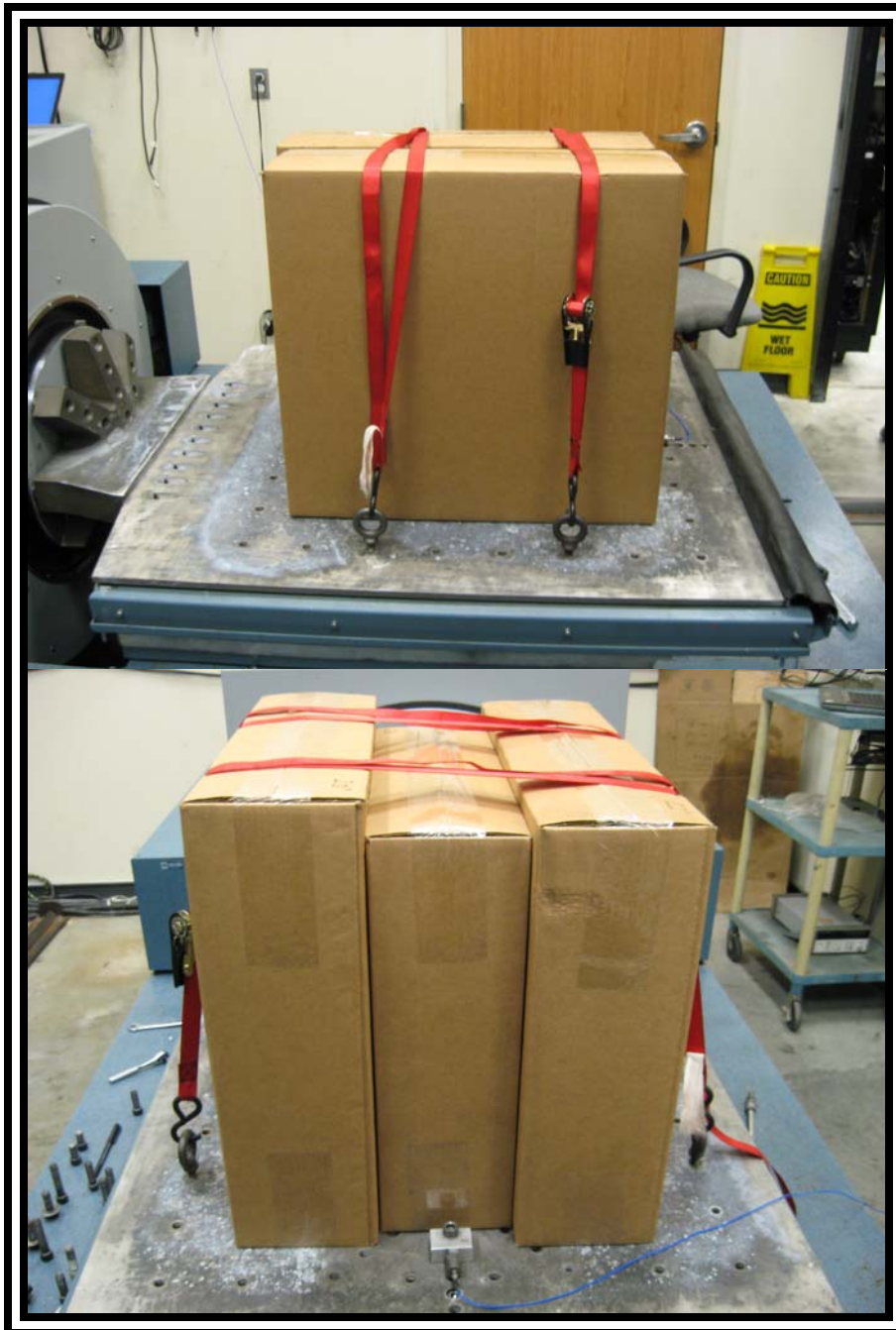
Figure 4: View of the test setup for Test 10 (random vibration)
