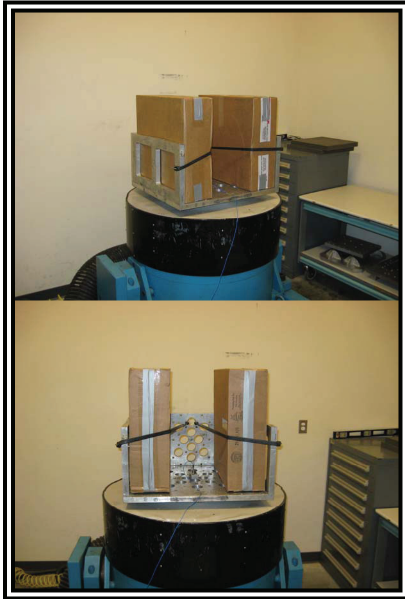
Figure 3: View of the test setup for Test 10 (random vibration)
