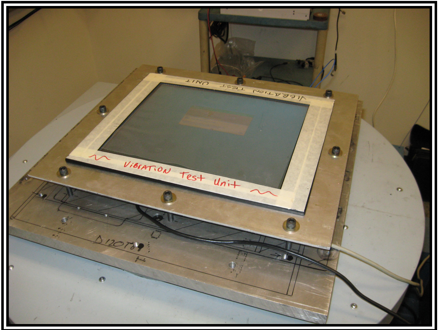
Figure 1: View of the test setup for Test 6 (mechanical shock) and Test 11 (sinusoidal vibration) Vertical Axis
