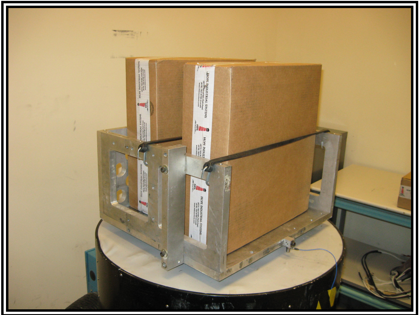
Figure 4: View of the test setup for Test 10 (random vibration) Horizontal Axes
