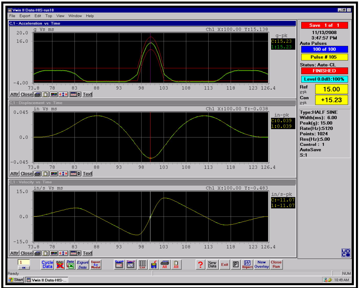
Figure 5: Time history of a representative shock pulse (15g, 6ms, ½-sine) Positive Direction
